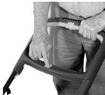
Figure 17. Pushing the Mower/Auxiliary switch to the Auxiliary setting
